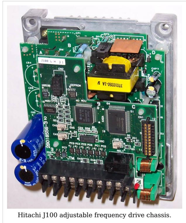
Hitachi J100 adjustable frequency drive chassis.
